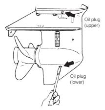
② Insert the oil tube nozzle into the lower oil plug hole, and fill with gear oil by squeezing the oil tube until oil flows out of the upper plug hole.
