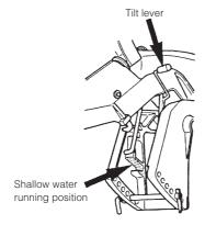
2 Return to normal running position: Tilt the outboard motor up fully and then return the outboard motor down slowly to the normal running position.
