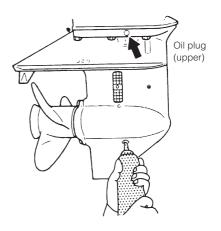
3 Install the upper oil plug, and then remove oil tube nozzle and install the lower oil plug.
